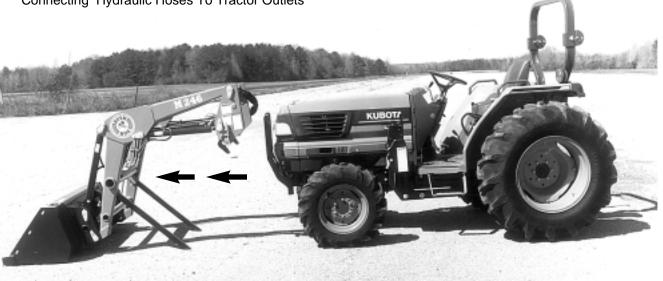
C. Check that lift cylinders are fully retracted. Figure 2-3. Then drive tractor forward. Use bucket cylinders to position height of outer pedestal top pin. Figure 2-4.
